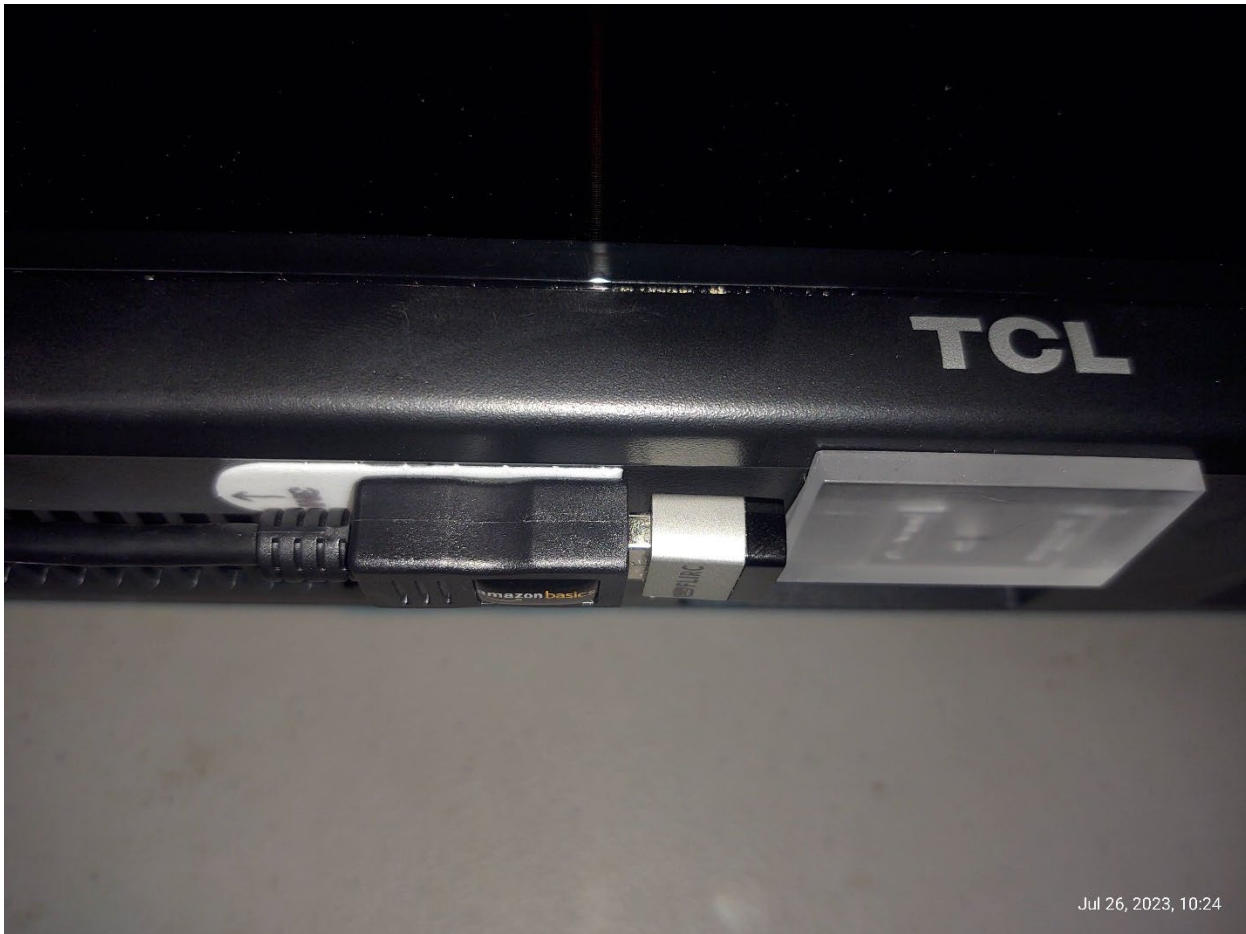
Figure 12 USB Extension cable w/ FLIRC attached to TV
