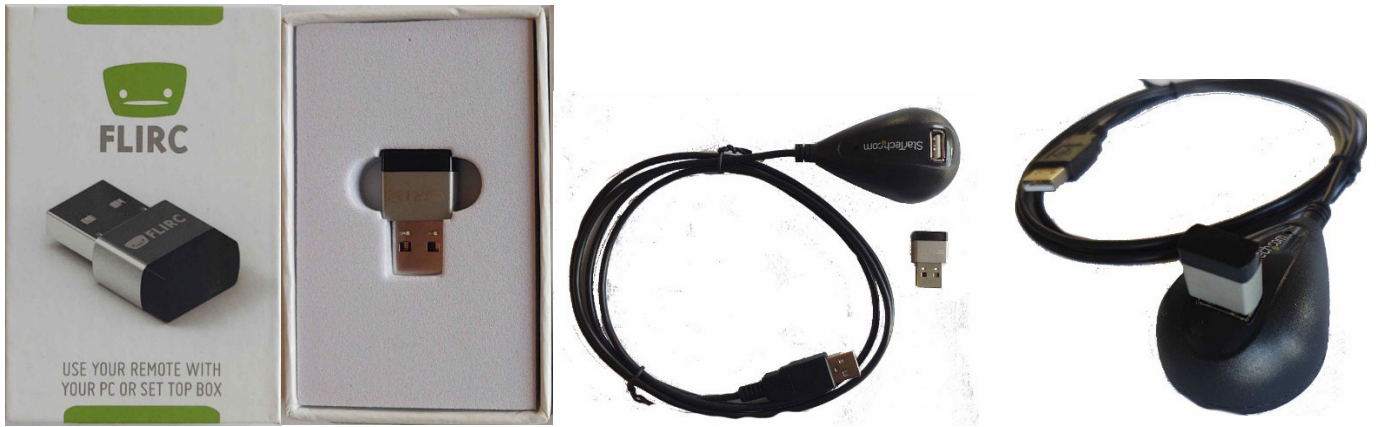
Figure 10 FLIRC inserted in Weighted USB Extension Cable
