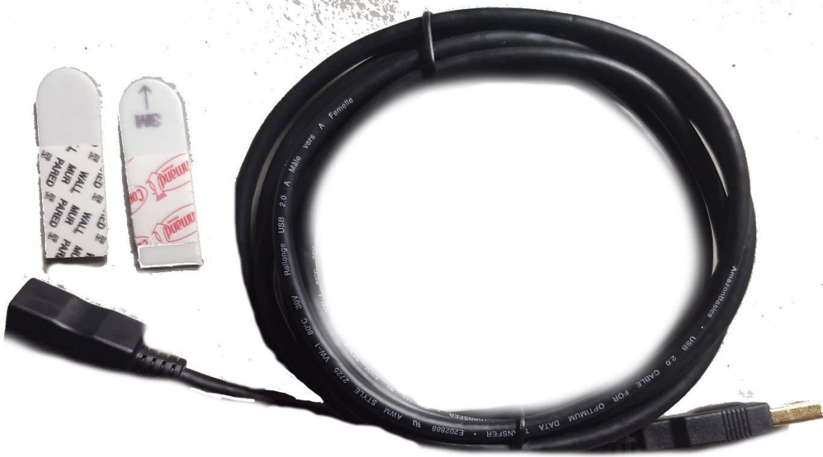
Figure 11 USB Extension cable with command strips (any double sided tape will do)
