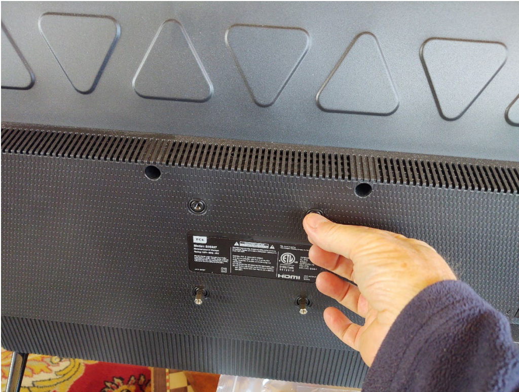
Figure 22 Insert Mounting Standoffs
