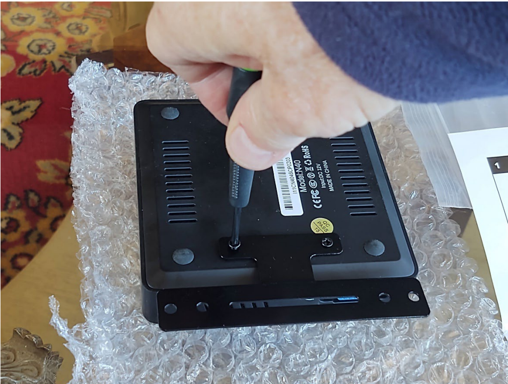
Figure 25 Install bracket on PC
